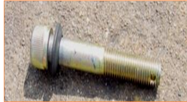
HEXAGONAL SOCKET HEAD CAP SCREW M16x100 mm (2 Nos )
