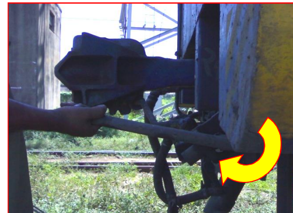
ROTATE OPERATING ROD IN CLOCK-WISE DIRECTION MINIMUM OF 90°
