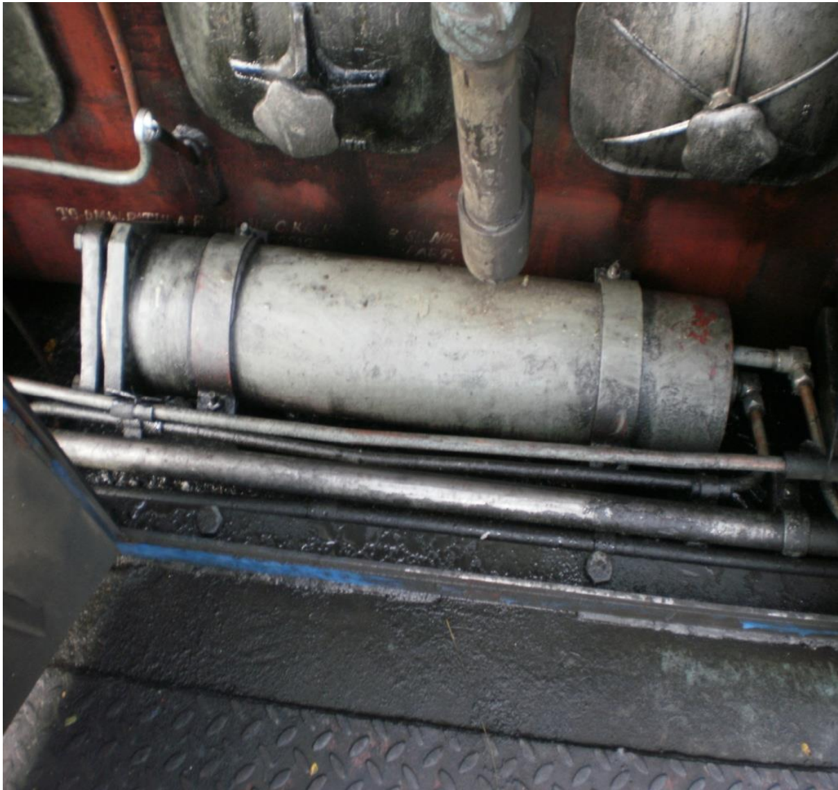
Primary Filter provided on right side of Engine Block in WDM3D Loco
