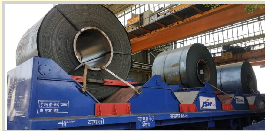
BFNV Rake: For damage free transport of steel coils
