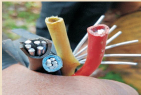
At Middle (@ 866m) : 4 x 95 sqmm - 06 strands in each core.
