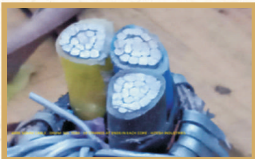
At Ends : 4 x 95 sqmm - 19 strands in each core.
