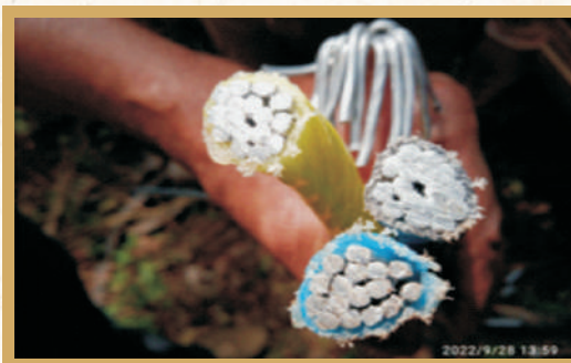
At Middle (@ 866m) : 4 x 95 sqmm - 16 strands in each core.
